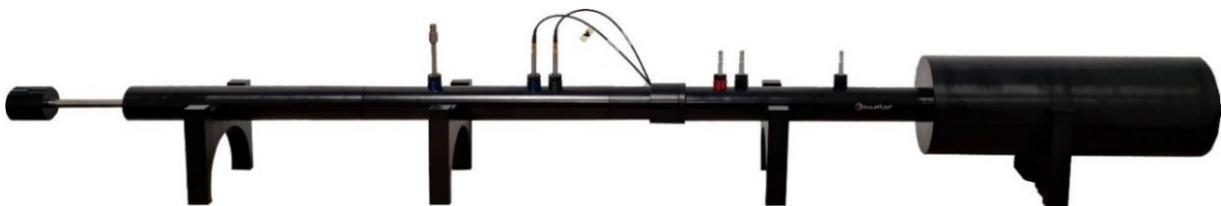
Figure 1. Impedance tube used for the measurements.
