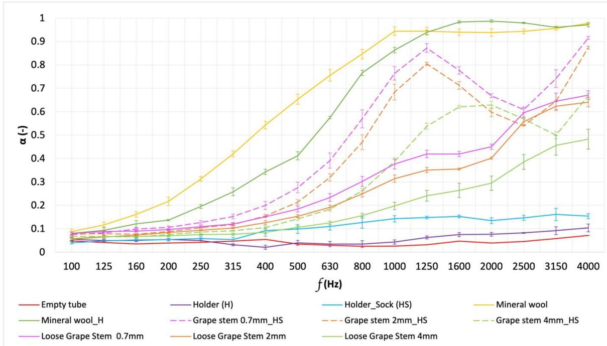
Figure 4. Comparison of frequency dependent sound absorption of tested variations.
