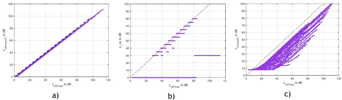
Figure 2. Correlation between single number rating approaches. a)  $L_{iAFmax} / L_{iAFmaxVT}$ ; b)  $L_{iAFmax} / L_{i-XX}$ ; c)  $L_{iAFmax} / L_{iFmaxAV}$ .
