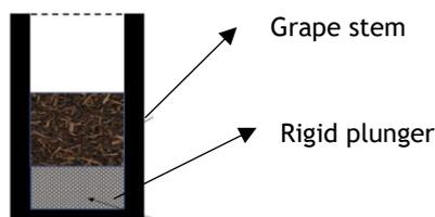
Figure 3. Illustration of the vertical impedance tube set-up.
