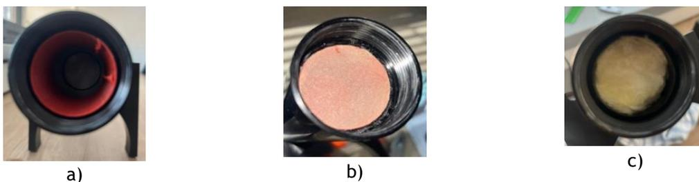
Figure 2. a) Holder b) Holder with sock c) Mineral wool.
