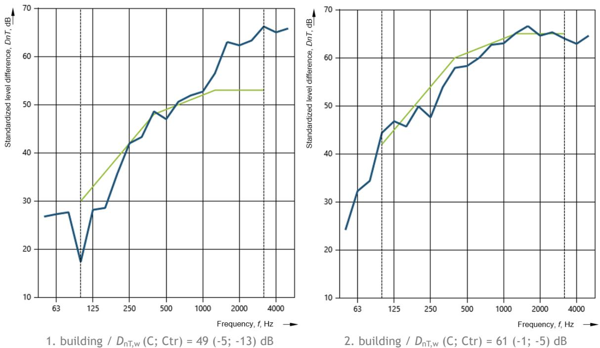
Figure 3. Graphs of the standardized level difference dependence on 1/3 octave band frequencies.
