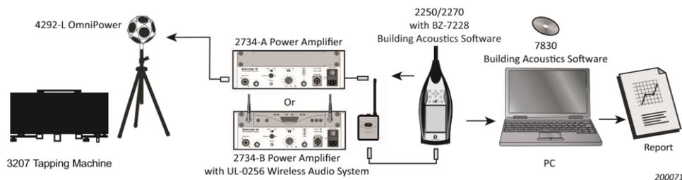
Figure 1. Schematic connection of equipment for measuring parameters of building acoustics from Brüel & Kjær (PRODUCT DATA: SOUND SOURCE AND IMPACT SOUND SOURCE FOR BUILDING ACOUSTICS, 2023).
