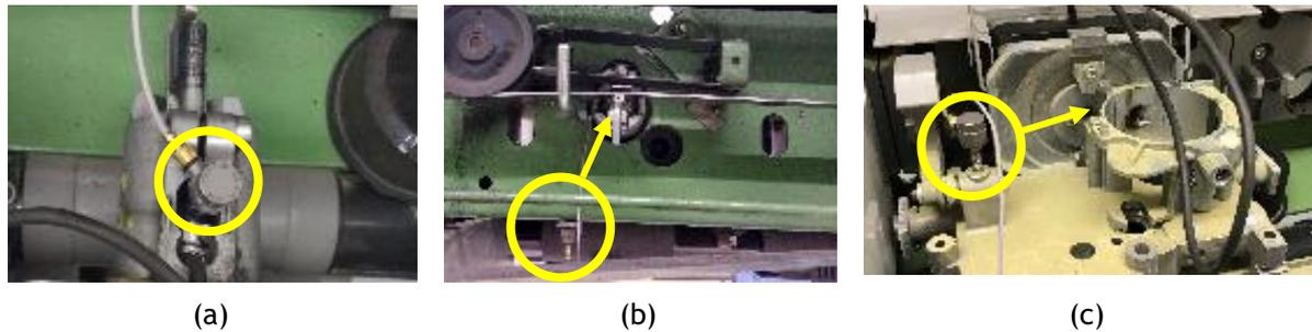
Figure 2. Different measurement locations of the accelerometers of the analysed bearing, (a) using a grub screw resting directly on the outer ring of the headstock bearing, (b) fixing with a magnet on the supporting frame of the drive unit under the analysed bearing and (c) on the spinning unit (frame) using a grub screw.
