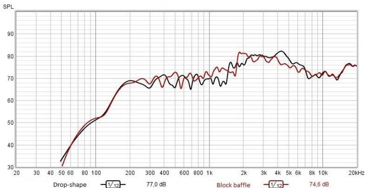
Figure 2. Comparison of frequency characteristics of loudspeaker enclosures.
