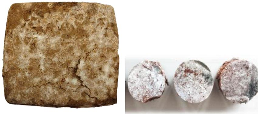
Figure 1. Mycelium composite and extracted samples for sound absorption and flow resistivity tests 45 mm diameter samples.
