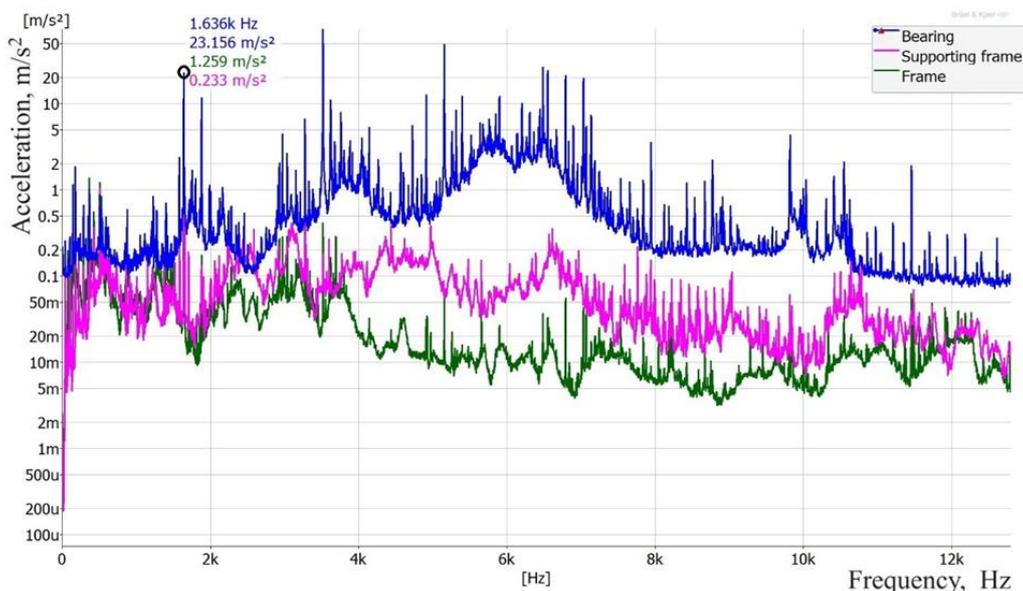
Figure 3. Frequency spectrum of the diagnosed bearing at the set rotation frequency of 100 000 r/min.
