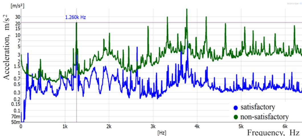
Figure 1. The bearing frequency spectrum of satisfactory and non-satisfactory spinning unit.
