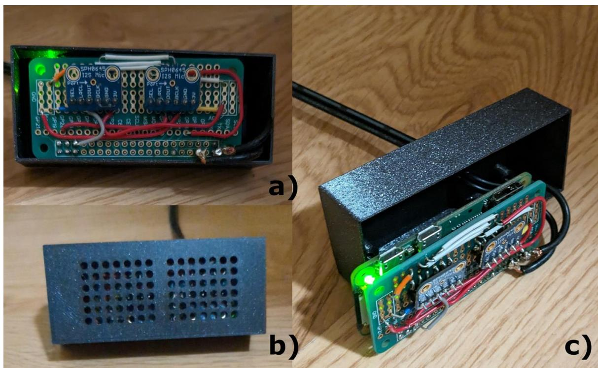
Figure 1. Photography of I2S microphones a) which are enclosed in the front panel b) are stacked on top of a Raspberry Pi Zero board (under the microphone plate) c).
