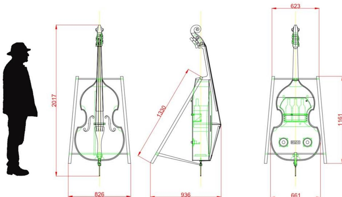
Figure 1. Basic dimensions of the special double bass and its comparison to average male figure.
