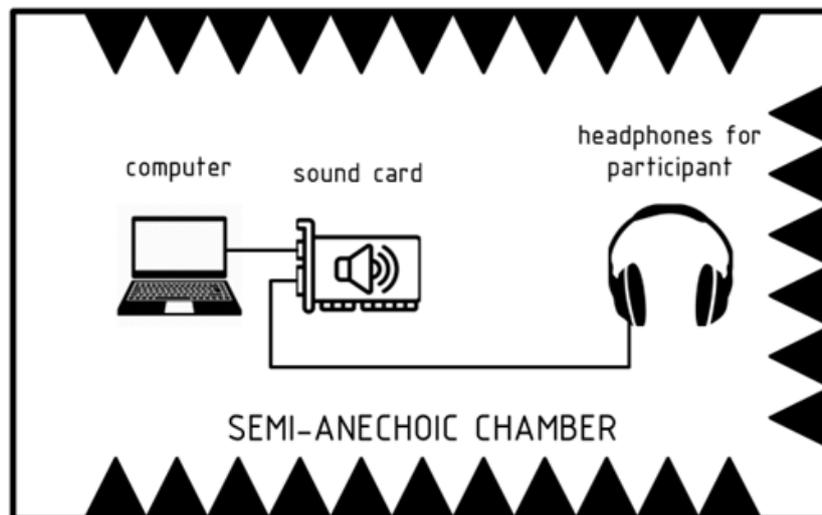
Figure 2: Setup scheme for the listening tests.
