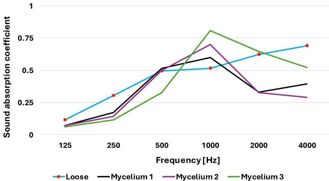
Figure 2. Sound absorption coefficient of coffee grounds and coffee ground based mycelium composites.
