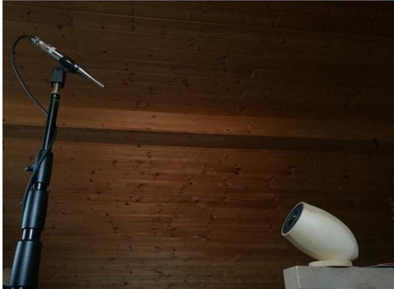
Figure 1. Measurement of loudspeaker system (Photo Jan Kozel).
