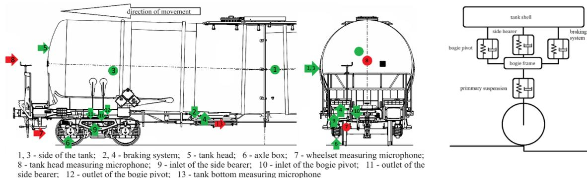
Figure 1. View of the distribution of accelerometers and microphones and schematic diagram of the transmission of vibration from the contact of the wheel with the rail to the shell of the tank.
