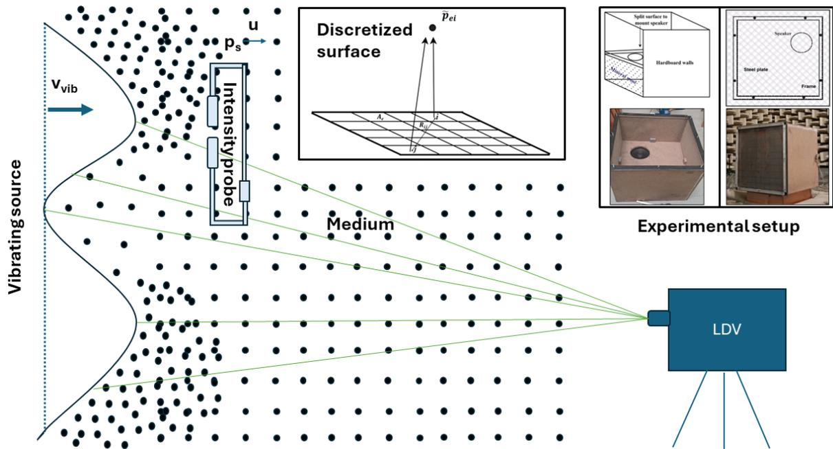
Figure 1. Sound pressure and surface velocity-based sound power determination.
