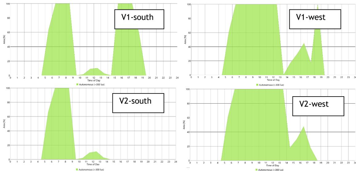
Figure 3. Calculation of sDA; comparison of the two strategies for different orientations (south and west), a percentage of the floor area exceeding 300 lux is shown.
