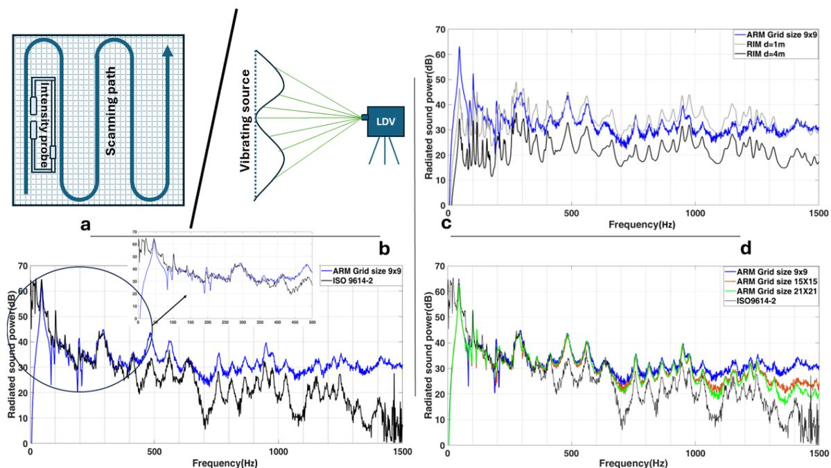
Figure 3: Sound power determination using acoustic pressure and surface velocity. a). Intensity probe and LDV measurement procedure, b). Comparison of ARM with ISO, c). Comparison of ARM with far and near field sound power using RIM, d). Effect of grid size on the accuracy of ARM.
