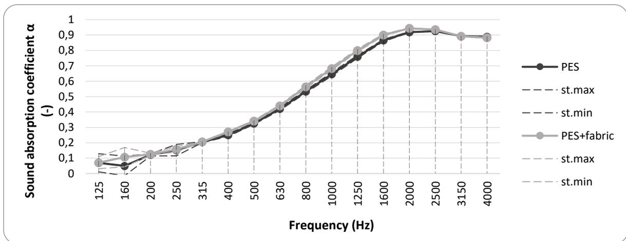
Figure 3. Sound absorption coefficient - PES fiberboard with and without the nylon fabric.
