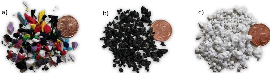
Figure 1. Investigated plastic granules: a) ethylene-vinyl acetate (EVA), b) polyethylene (PE), c) polystyrene (PS).
