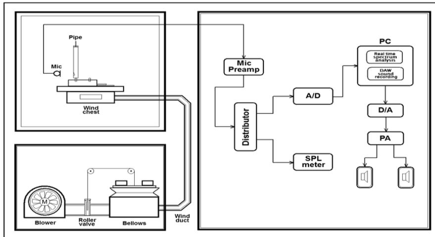
Figure 1. Measurement apparatus scheme.
