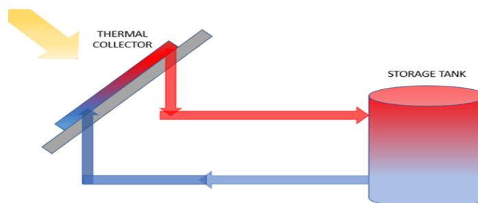
Figure 1. Block diagram of solar thermal collector and storage tank.
