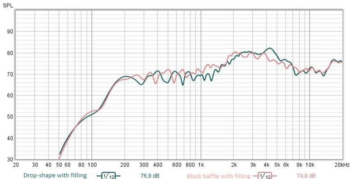
Figure 3. Comparison of frequency characteristics of loudspeaker enclosures with filling.
