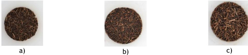
Figure 1. Grape stem by-products obtained a) 0 - 0.7mm, b) 0.7 - 2mm, c) 2 - 4mm.
