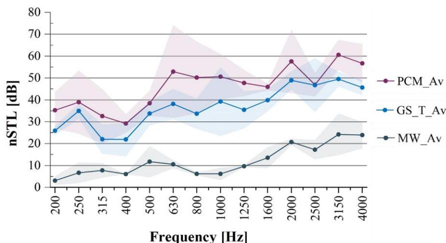
Figure 3. The normal Sound Transmission Loss (nSTL) obtained for the analysed samples, together with the standard deviations of the results.
