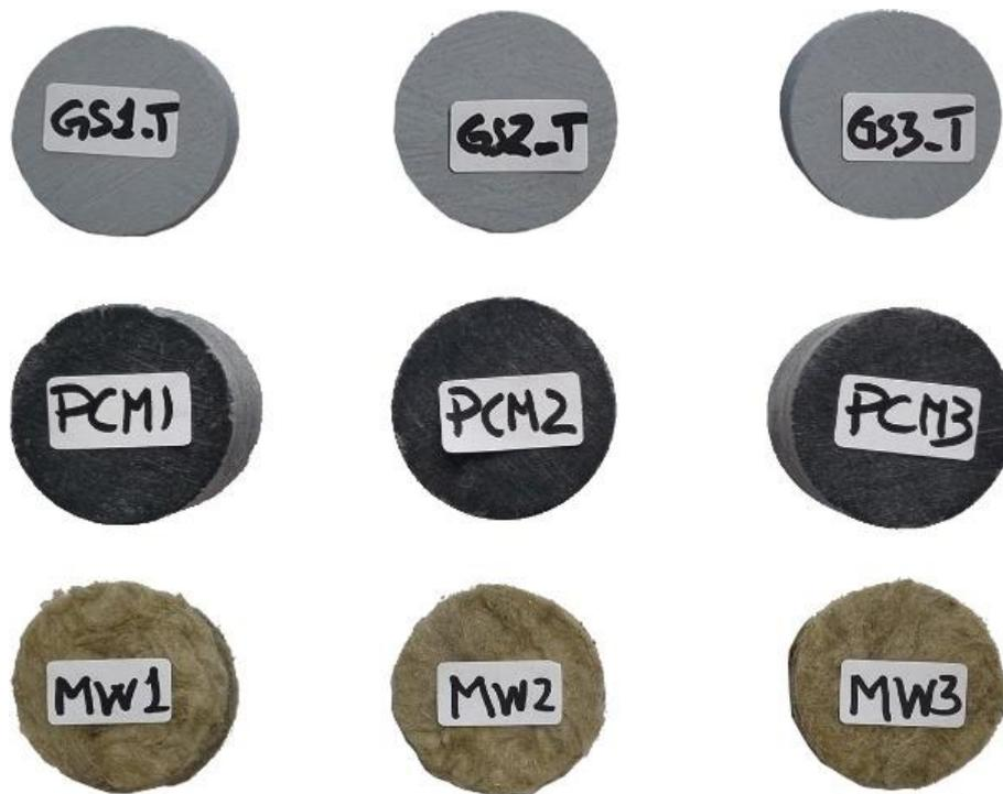
Figure 2. Samples used for the impedance tube measurements.
