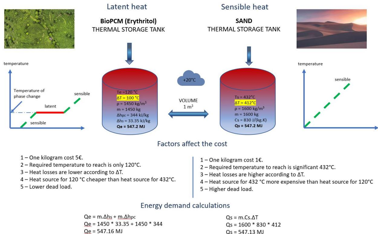
Figure 2. Analyses and comparison between PCM tank (LHS) and sand tank (SHS).
