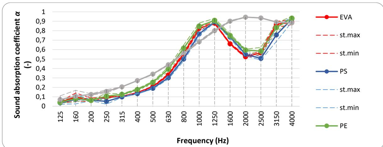
Figure 4. Sound absorption coefficient of porous granulated plastic materials.
