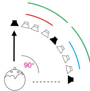
**Obf. 1:** Experimental setup for the Exp. 3. Black loudspeakers indicate possible distractor locations (only one distractor location was used in each experimental run), while target could be presented from each of the 7 inner loudspeakers (in target-alone-trial targets) or was restricted to specific subregion of the speaker array (in contextual trials) in left-half/right-half/full-context condition (coded here and in other Exp 3&4 figures by red, blue and green color , respectively).
